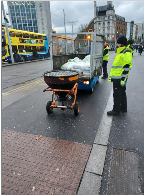
Photograph 5. WMS using their motorised refuse cart with mini-gritter being towed
