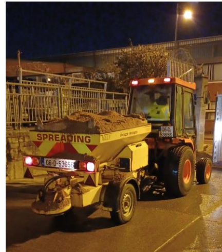
Photograph 2. RMS tractor ready for gritting cycle lanes
